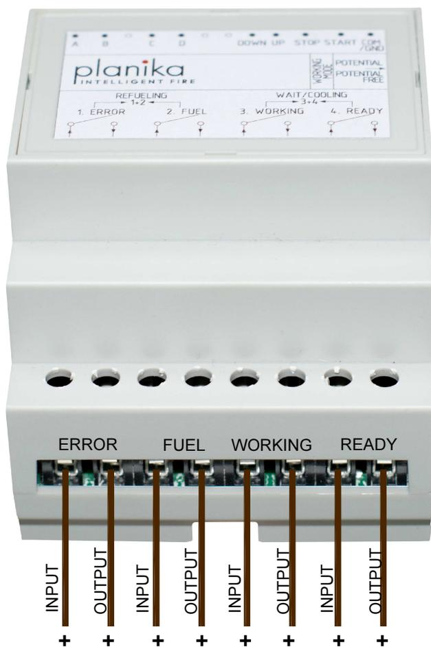
INPUT – voltage signal input, from 12V to 24V DC
